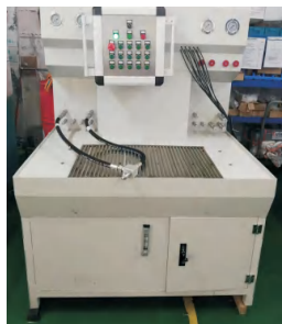
Valve Manifold Testing
